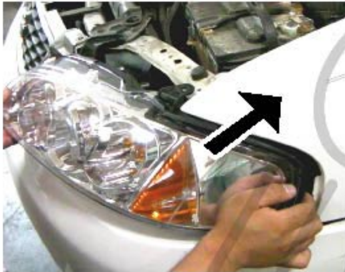
13. Put the headlight to the original spot
