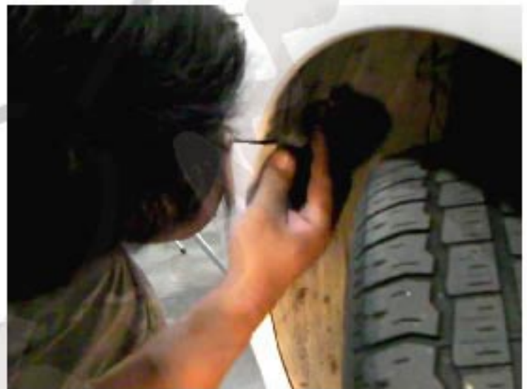
2. Remove one screw from the inside of the wheel well
