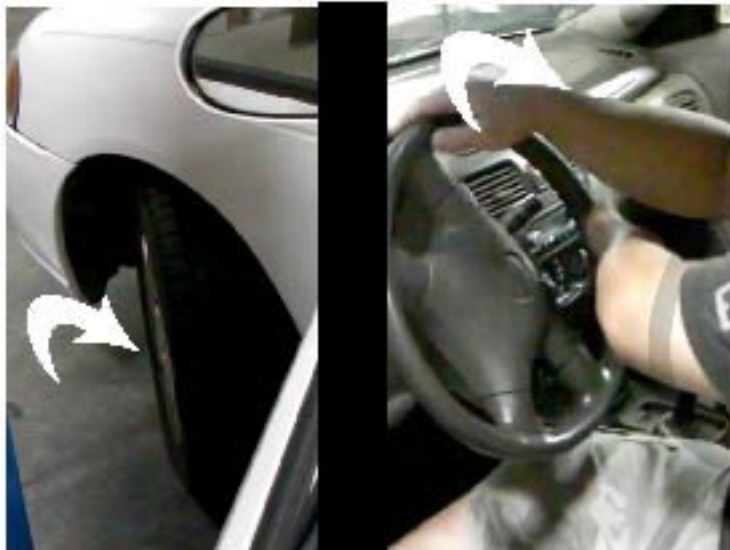
1. Space steer front wheels to the right
