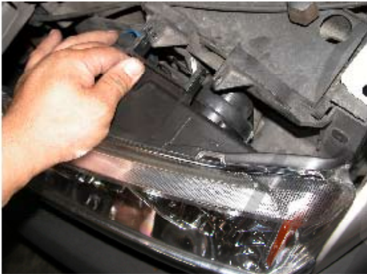
7. Gently install the headlight to its original spot
