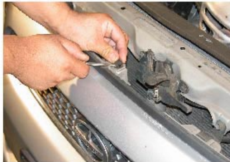
22. Install five clips on top of the grill (Please repeat the picture order from 1 to 22 for the opposite side)
