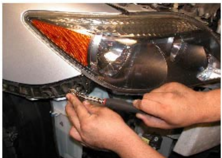
10. Remove one 10mm headlight bolt at side of the headlight
