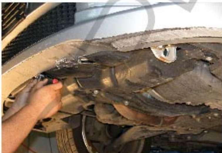
21. Install seven 10mm bolts under the front bumper
