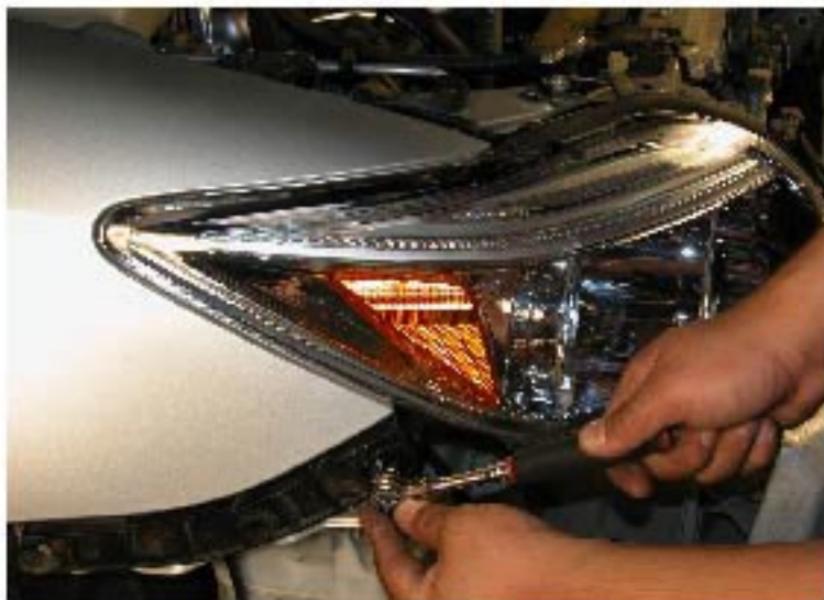
17. Install one 10mm headlight bolt on the side of the headlight
