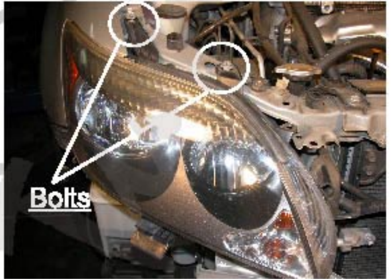
8. Two 10mm headlight bolts at top of the headlight
