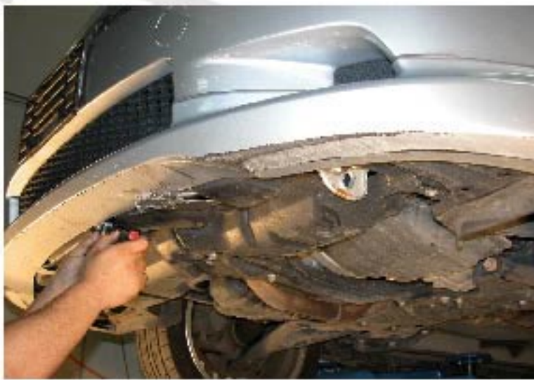
4. Remove seven 10mm bolts under the front bumper
