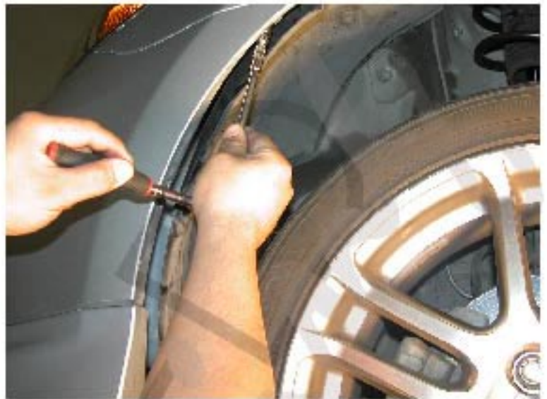
6. Then pull out the plastic cover just enough to see the 10mm bolt. Remove the 10mm bolt at side of the bumper (Both sides)
