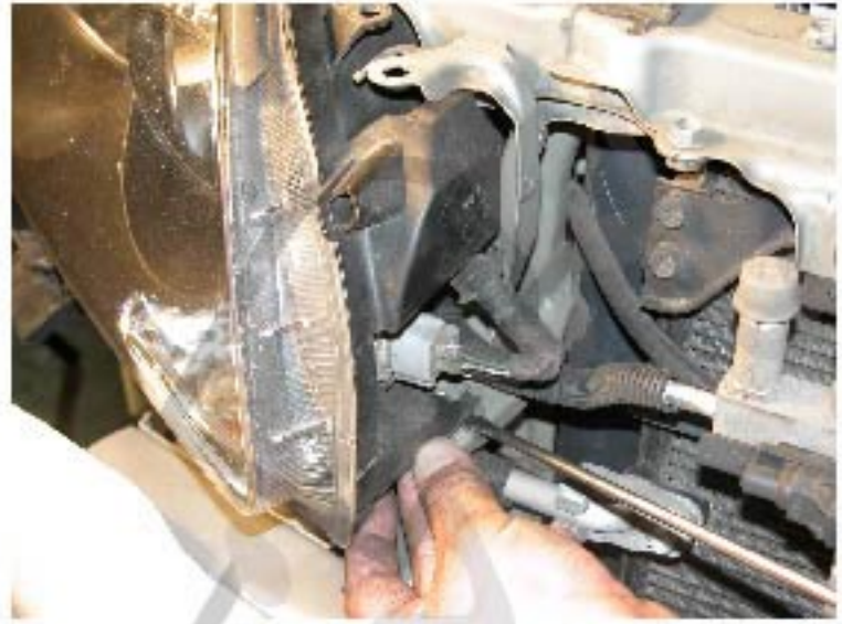
12. Unlock the headlight on the front corner
