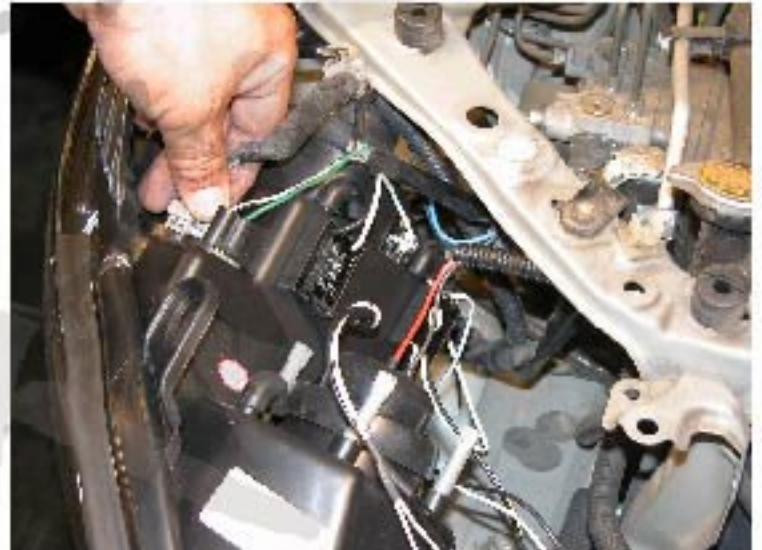
14. Connect all headlight connectors please see the "Halo and L.E.D. installation instructions" If your headlights don't have HALO or L.E.D. You can skip the installation instructions.
