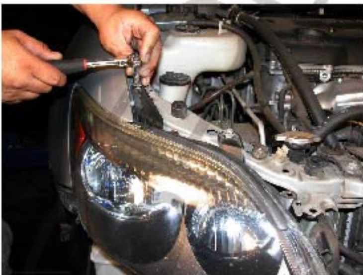
9. Remove two 10mm headlight bolts at top of the headlight
