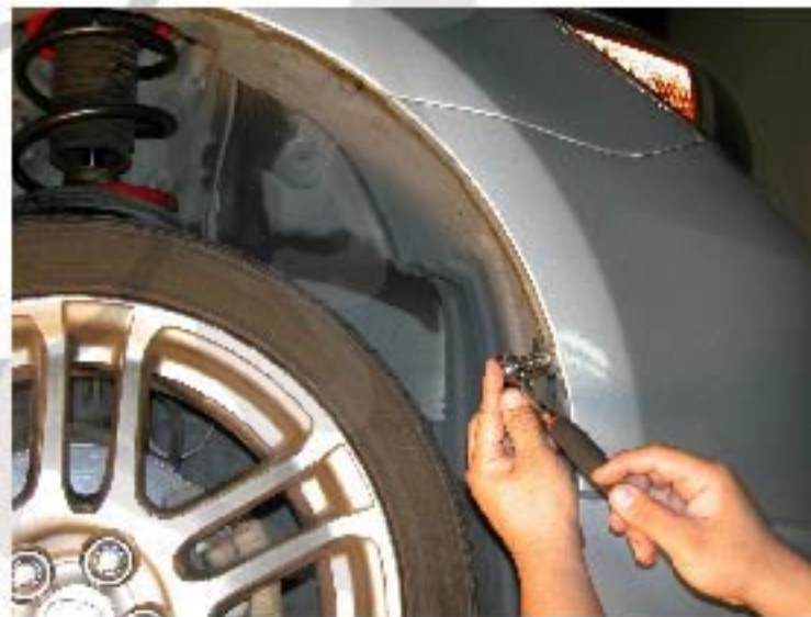
20. Install one 10mm bolt at the side of the bumper ( Both sides)
