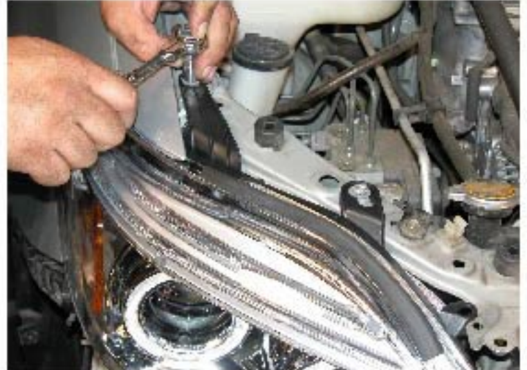
16. Install two 10mm headlight bolts at top of the headlight
