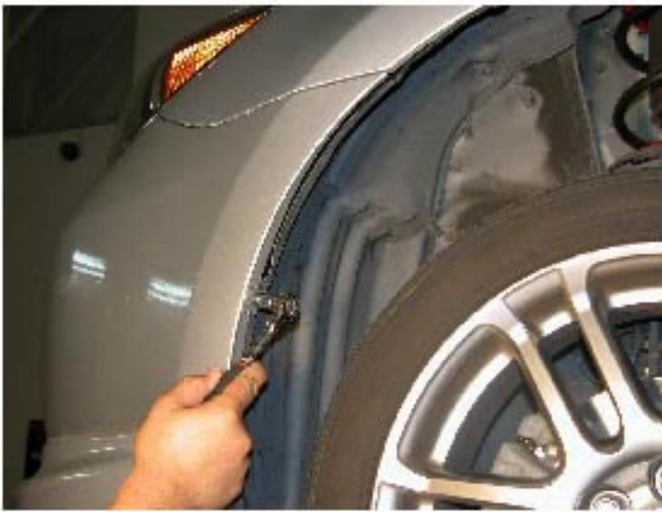
5. Remove one 10mm bolt at the side of the bumper first (Both sides)
