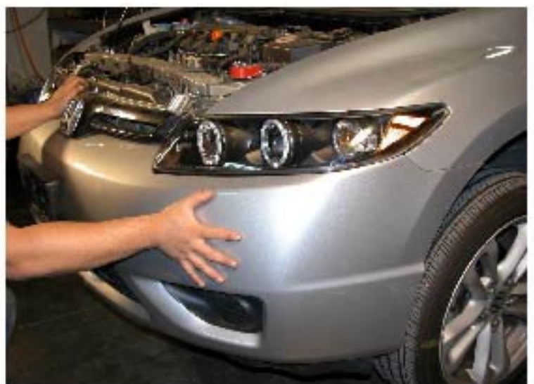
22. Install the front bumper
