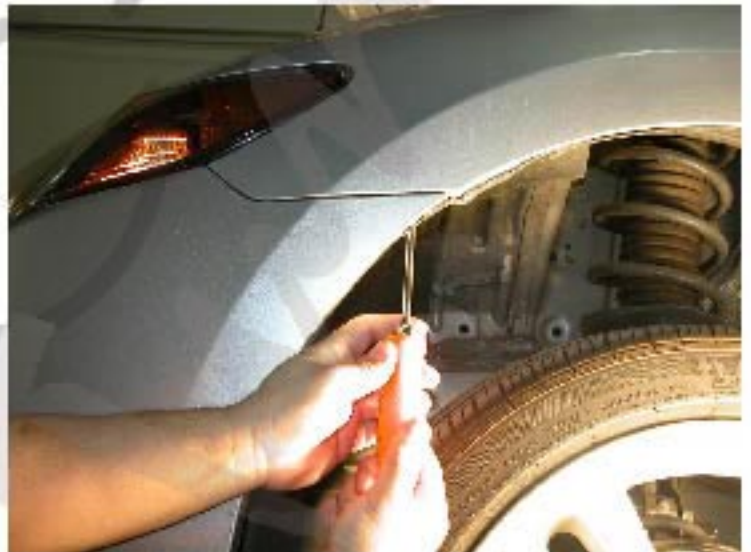
8. Remove one bolt at side of the bumper ( Both side)
