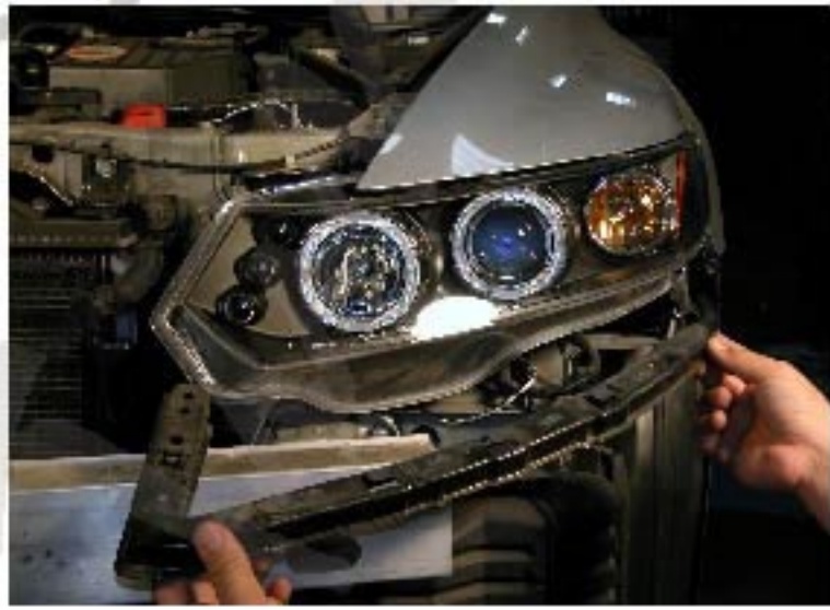
20. Install the bracket under the headlight
