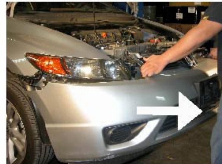
10. Remove the bumper slightly
