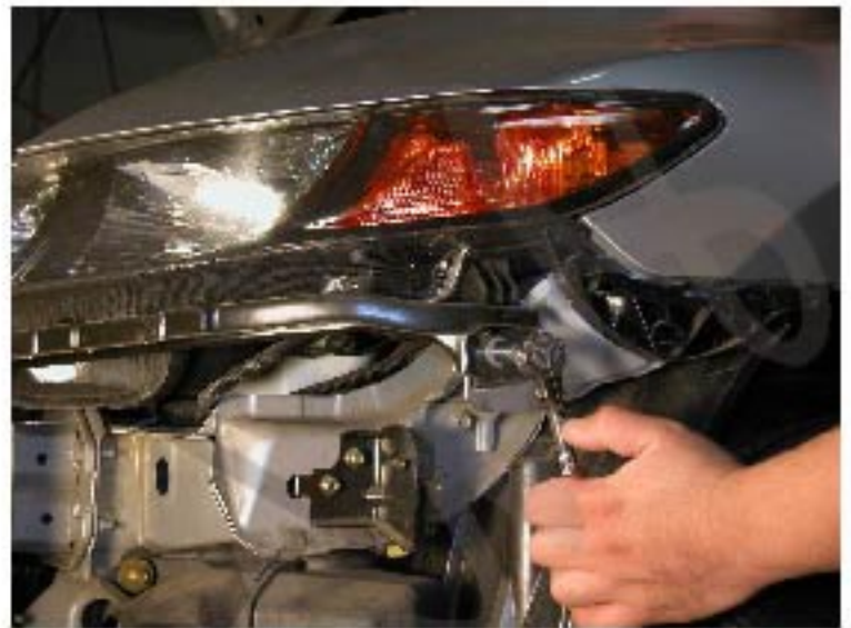
12. Remove one 10mm headlight bolt at side of the headlight
