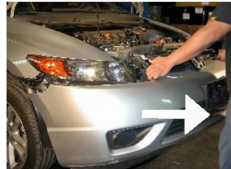
10. Remove the bumper slightly
