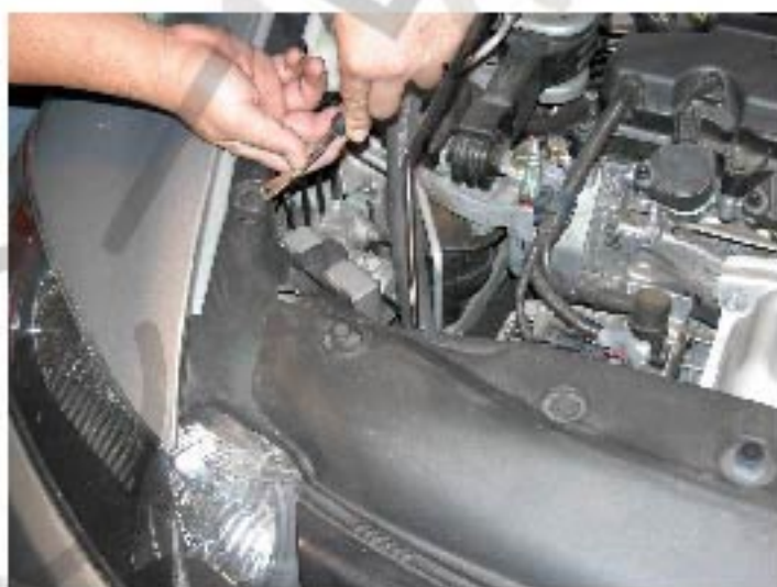
2. And then remove the four clips from the top of the grill
