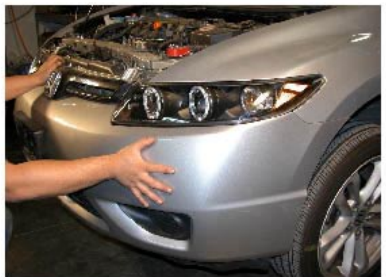
22. Install the front bumper
