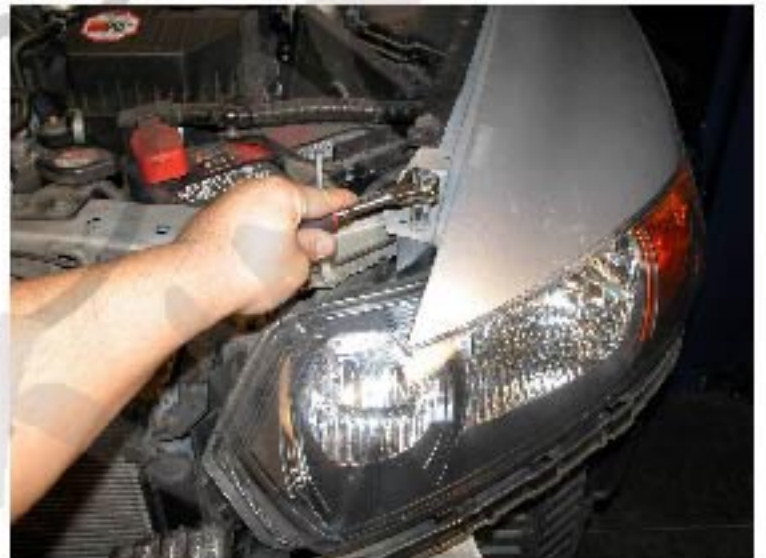
14. Remove two 10mm headlight bolts on the top of the headlight
