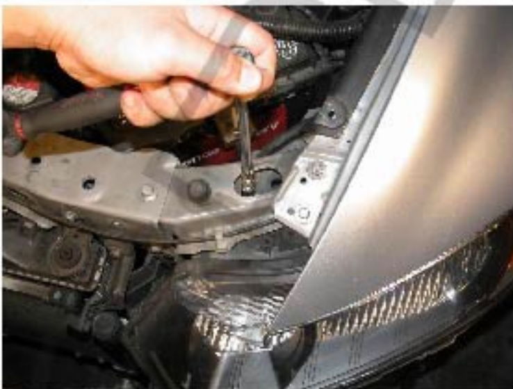
15. Remove two 10mm headlight bolts on the top of the headlight
