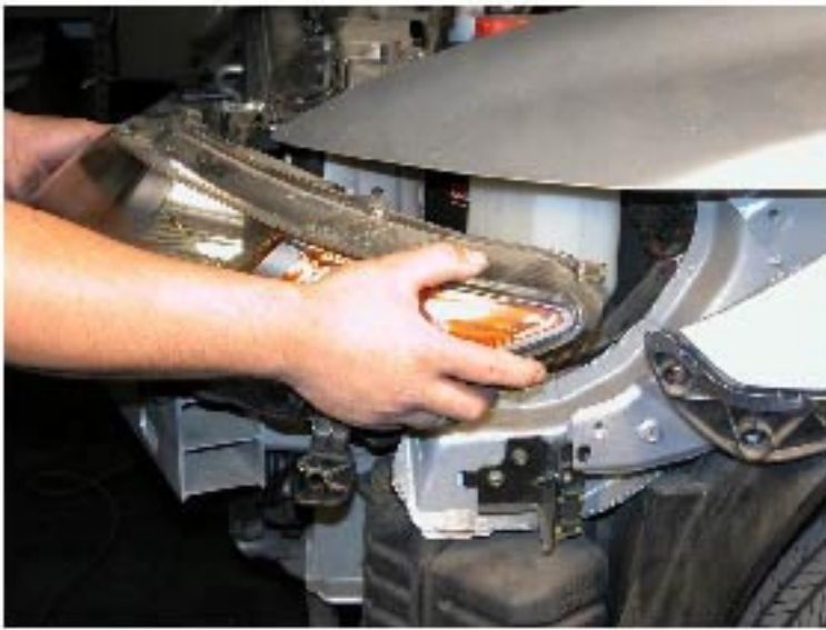
17. Remove the headlight
