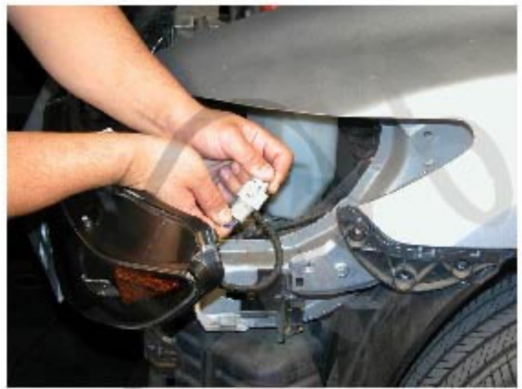
18. Install all headlight connectors please see the "Halo and L.E.D. installation instructions" If your headlights don't have HALO or L.E.D. You can skip the installation instructions.
