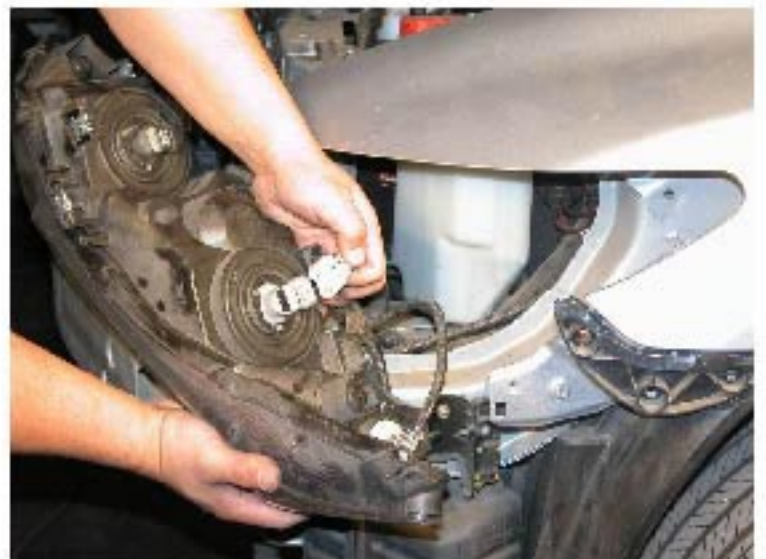
16. Disconnect all connectors from the headlight
