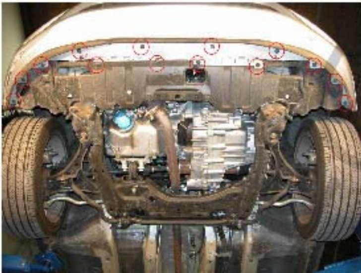
7. Remove fourteen clips under the bumper
