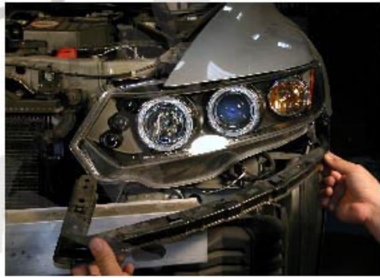
20. Install the bracket under the headlight
