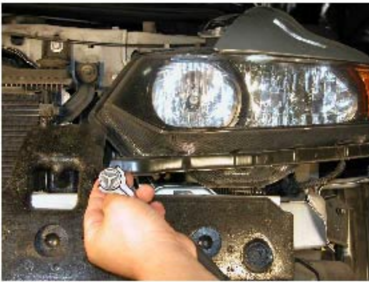
11. Remove one 10mm headlight bolt under the headlight
