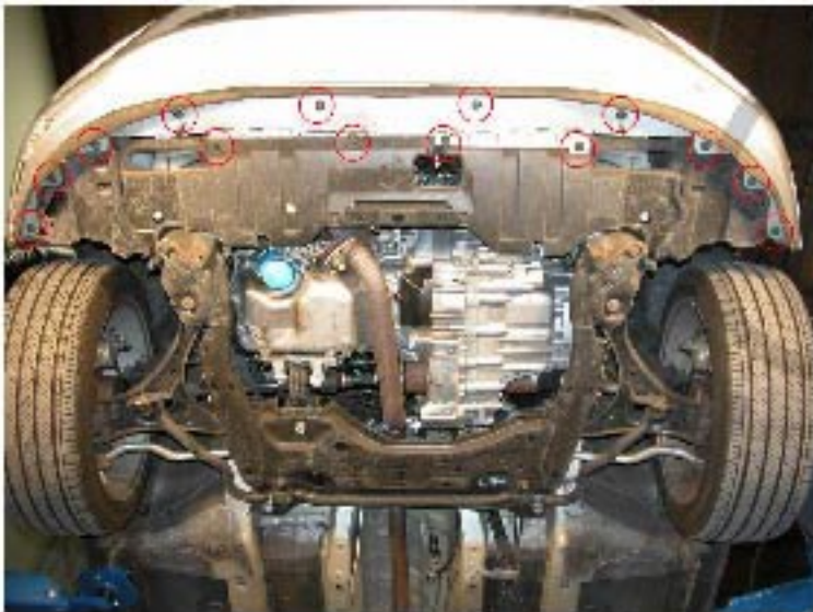
25. Install fourteen clips under the bumper
