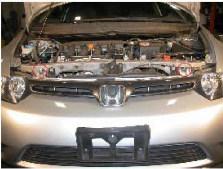
5. There are two bolts needed to be removed
