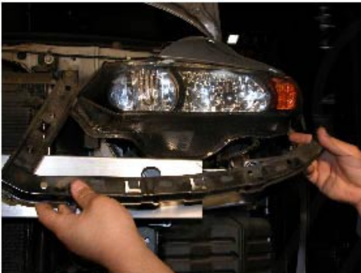
13. Remove the bracket under the headlight
