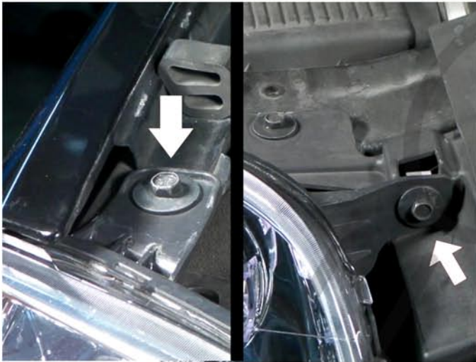
13. Install two bolts to fasten the headlight
