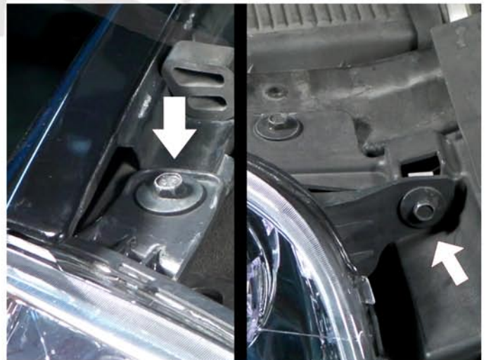
4. Remove two headlight bolts
