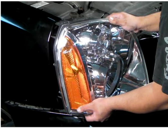
5. Pull out the headlight a little bit, just enough to see the wire harness in the back
