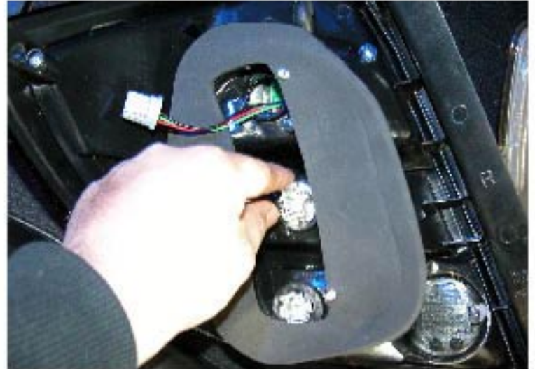
10. Plug all the sockets into the new L.E.D. tail light
