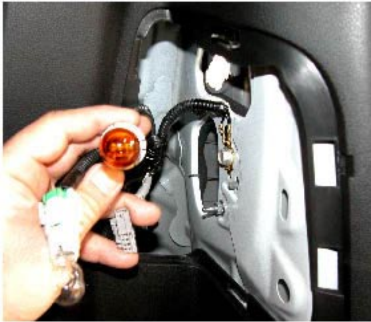
5. Pull out all the wires and connectors from the vehicle
