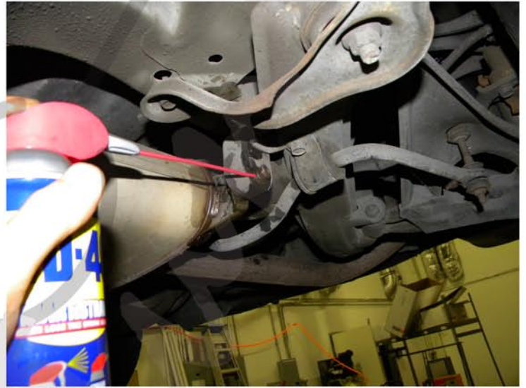
2. Spray the 12mm bolt with penetrating oil
