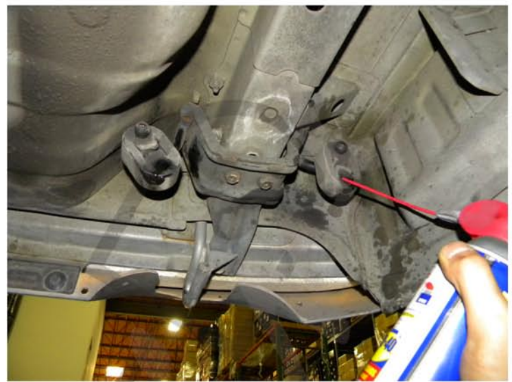
18. Spray the rear rubber exhaust hangers with penetrating oil
