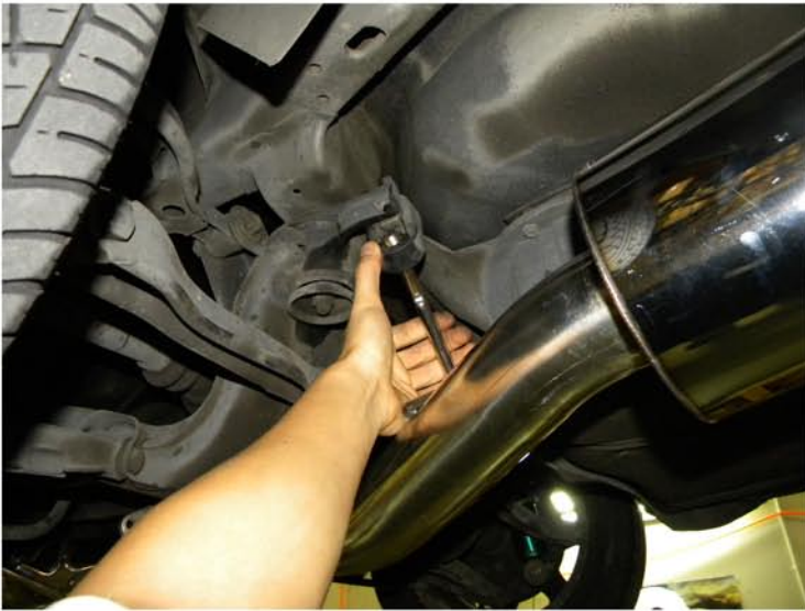
23. Slide the muffler section into the rubber hanger
