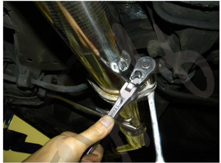
24. Tighten the 14mm nut and bolt connecting the front section and rear muffler section
