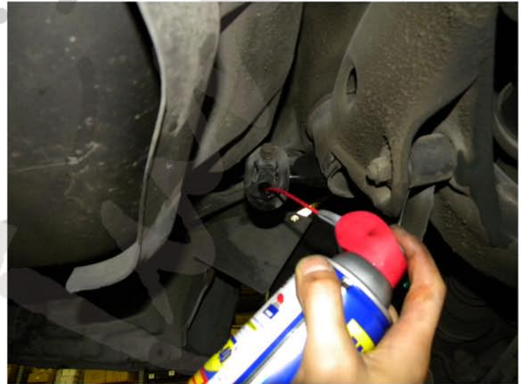
20. Spray the rubber exhaust hanger with penetrating oil
