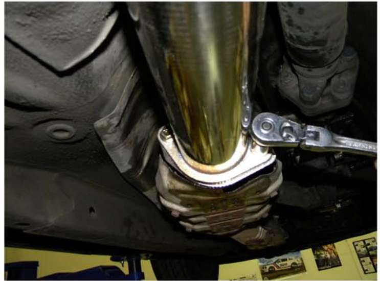
16. Tighten the 14mm bolt onto the catalytic converter
