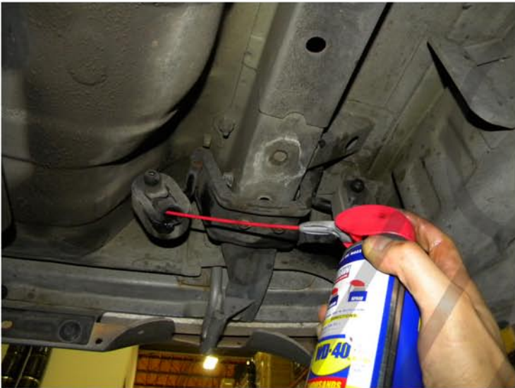
19. Spray the rear rubber exhaust hangers with penetrating oil
