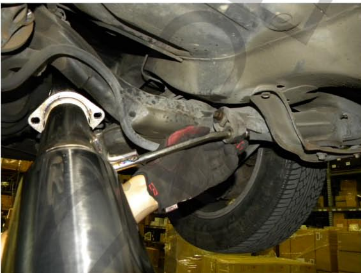
15. Slide the front exhaust section into the rubber hanger
