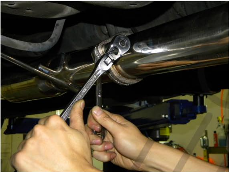
25. Tighten the 14mm nut and bolt connecting the front section and rear muffler section
