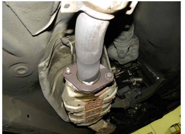
4. 14mm bolt and 17mm nut location
