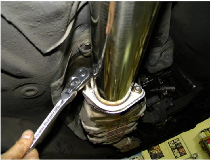
17. Tighten the 17mm bolt onto the catalytic converter
