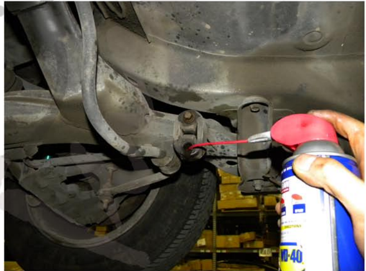
14. Spray the rubber hanger with penetrating oil
