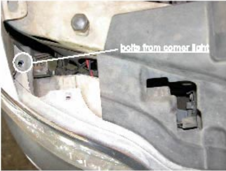
11. Install the bolt from corner light (BOTH SIDE)
