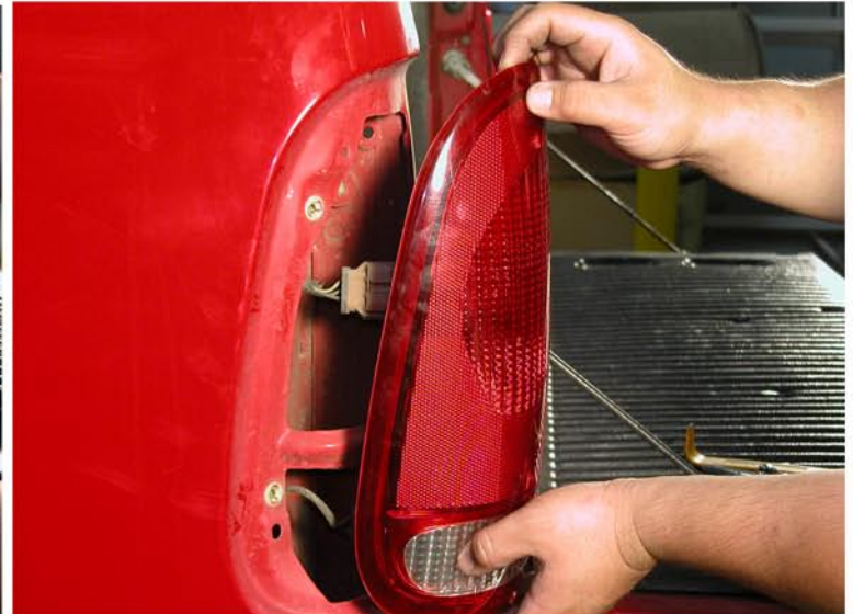
4. Pull out the tail light slightly, just enough to see the back of the tail light
