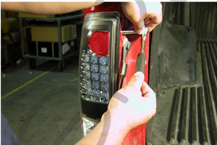
9. Install the two bolts to stabilize the tail light (Please do the other side follow the picture order from 1 to 9 )
