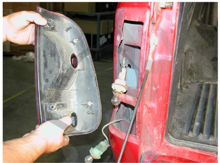
6. After disconnecting all the connectors, remove the OEM tail light
