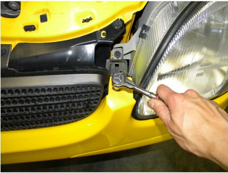
5. Remove the (2) 10mm bolts
