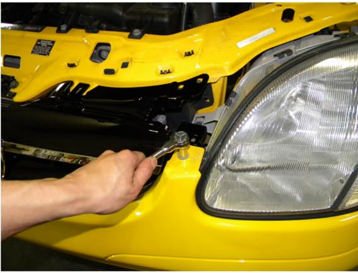
11. Tighten the (2) 10mm bolts
