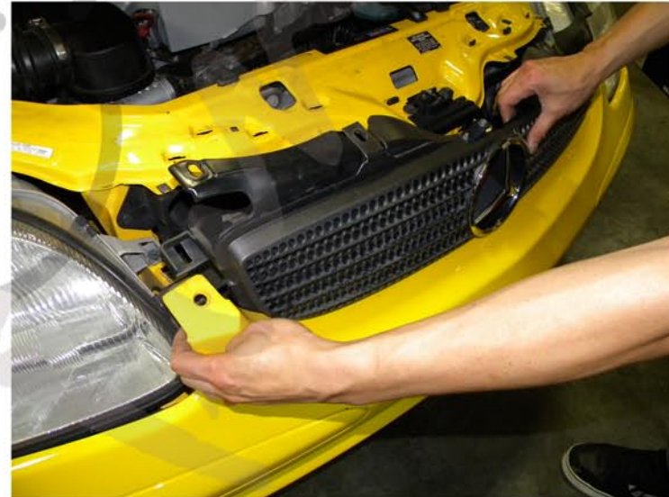
8. Pull on top of the front bumper
