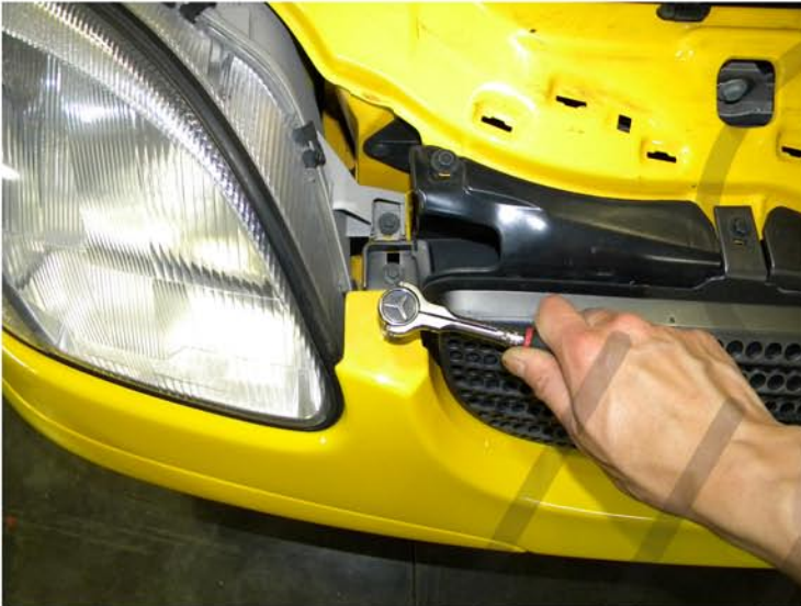
7. Remove the (2) 10mm bolts
