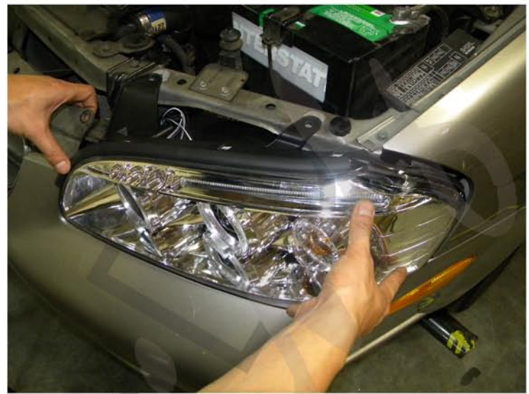
6. Make sure the new projector headlights are secure
