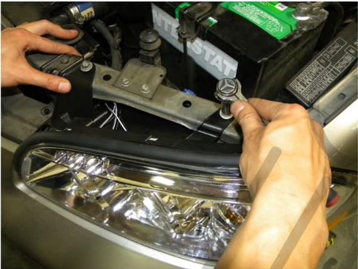
7. Screw back the two 10mm headlight bolts
