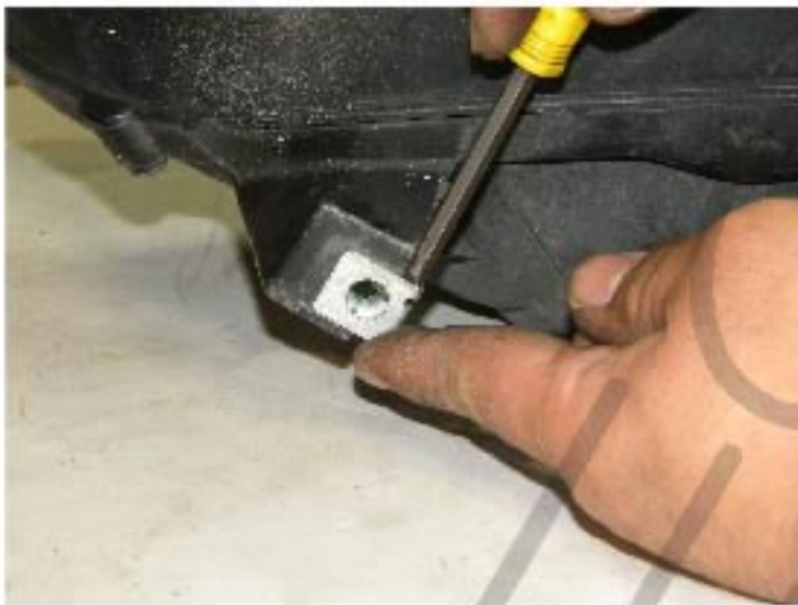
25. Remove the clip from the old headlight to the new headlight (both side)
