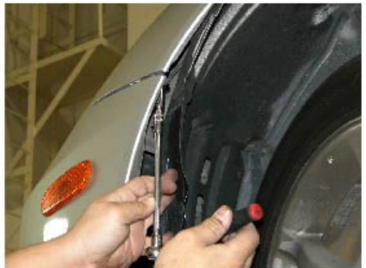
33. Install one bolt at side of the bumper (Both side)
