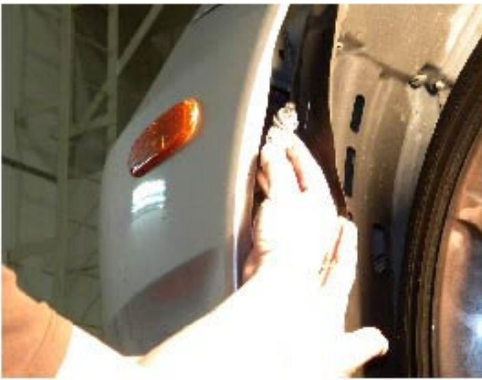
34. Connect driving light socket (side marker)
