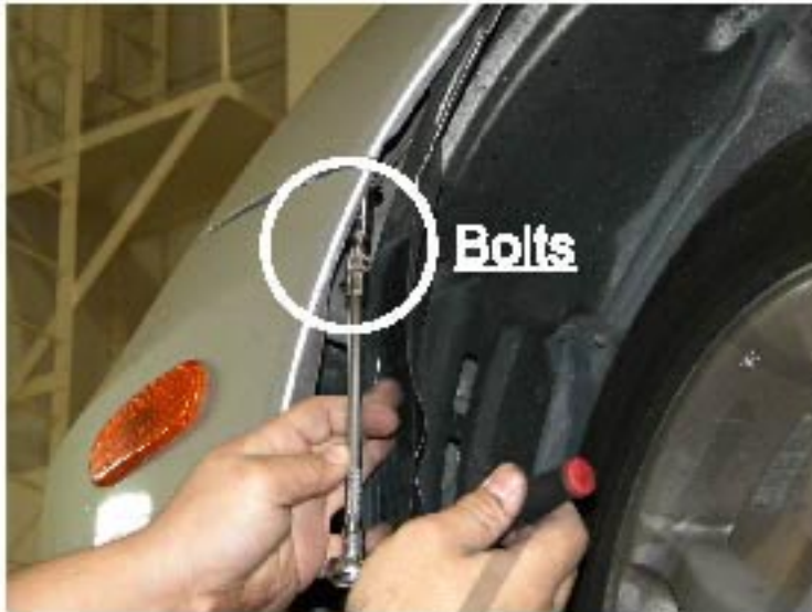
7. Remove one bolt at side of the bumper ( Both side)
