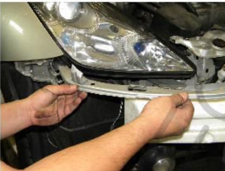
13. Remove the bracket under of the headlight
