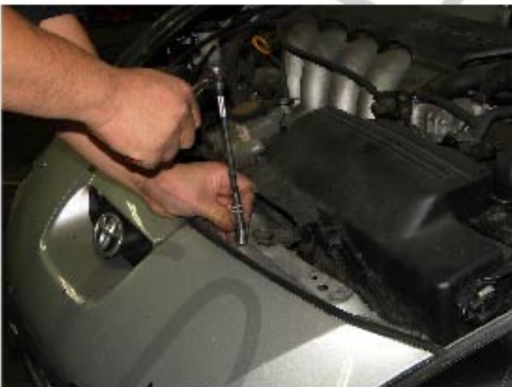
32. Install four bolts and one clip on top of the bumper
