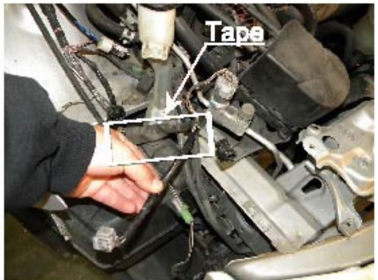
22. Cut and open the tape for protection the wires, so the wire can be longer to use
