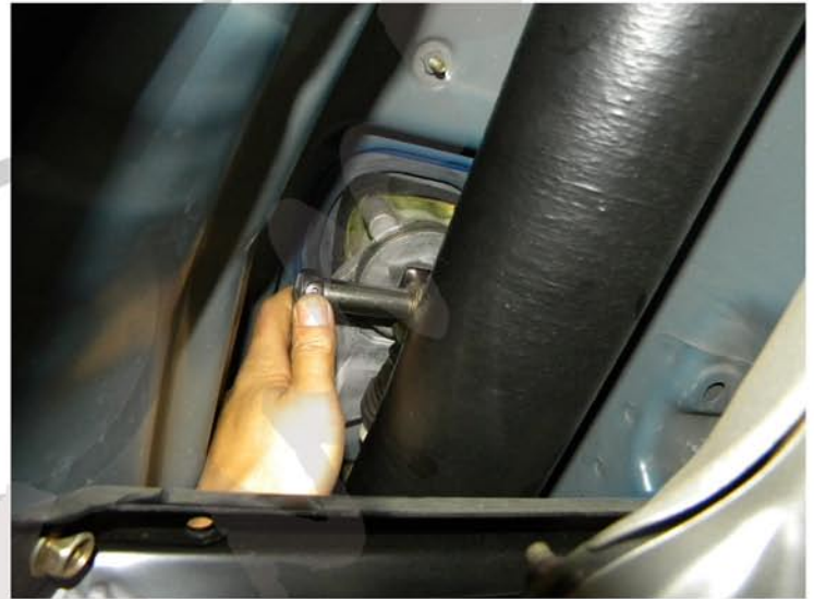
2. Remove a 12mm bolt connecting the short shifter and the shift link
