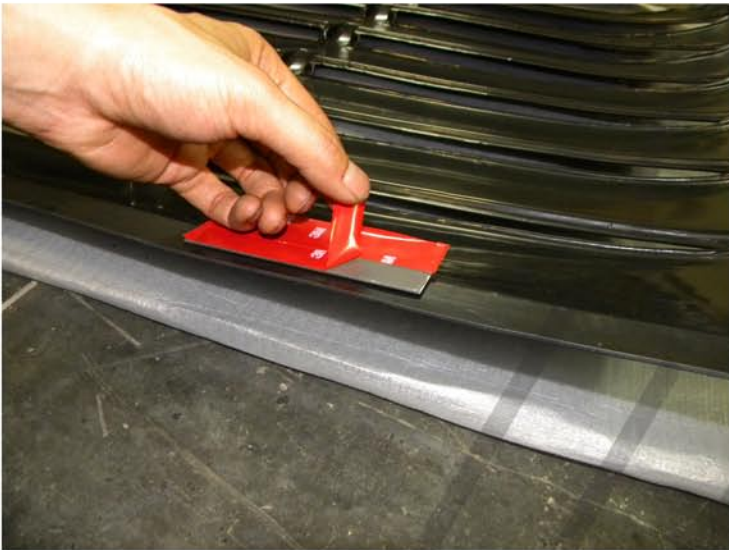
7. Peel off the tape backing on mounting brackets
