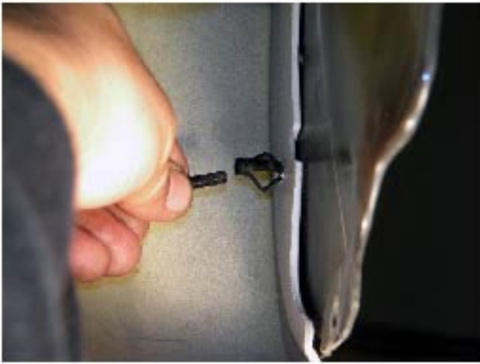
11. Pull out the screw inside the bumper
