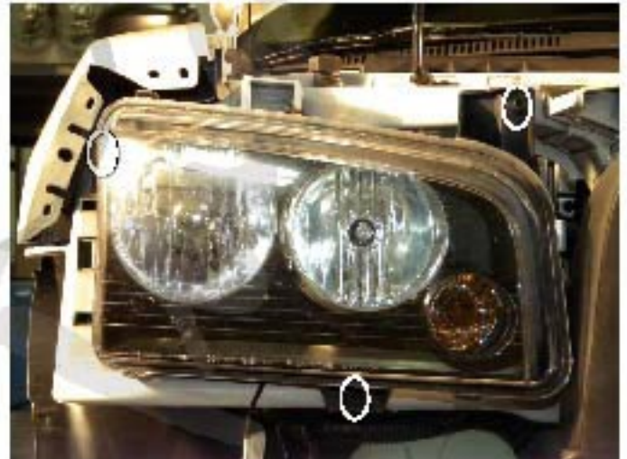
20. Remove three headlight bolts
