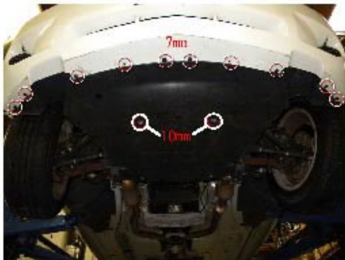
5. Remove ten 7mm bolts and two 10mm bolts
