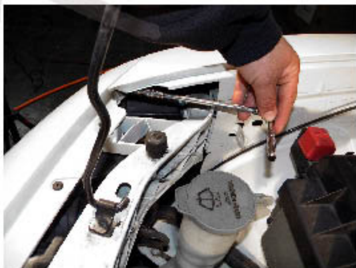
4. Remove one 10mm bolt by using 1/4" drive ratchet(Both side)
