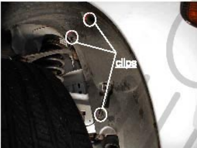
13. Remove three clips (Both side)
