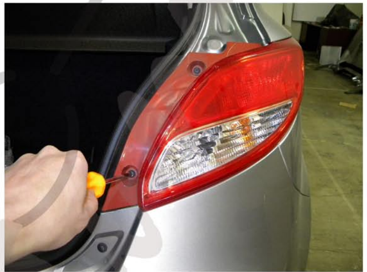
2. Remove the (2) phillips head screws
