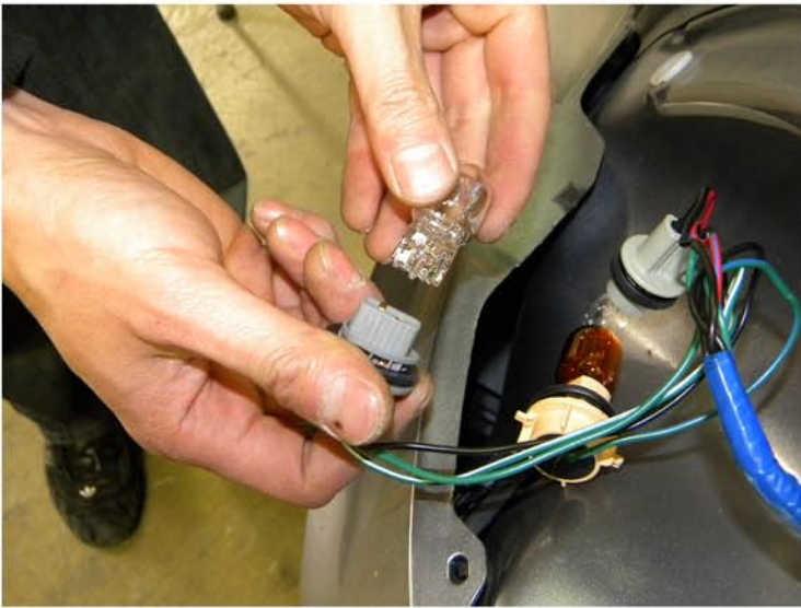
5. Remove the brake light bulb from the socket
