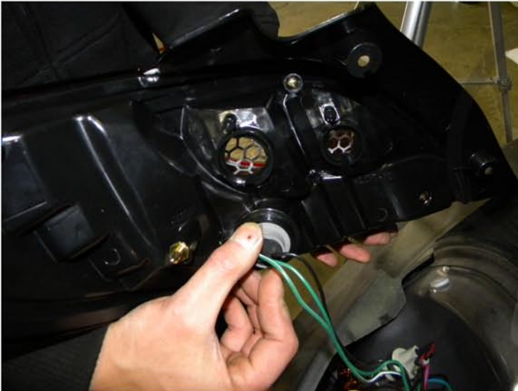
7. Place the light sockets in the LED tail light
