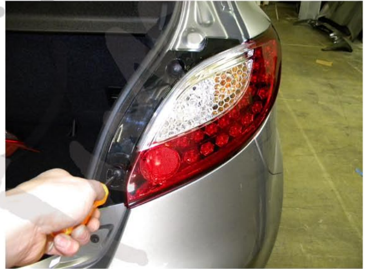
8. Place the LED tail light in stock location and tighten the (2) phillips head screws
