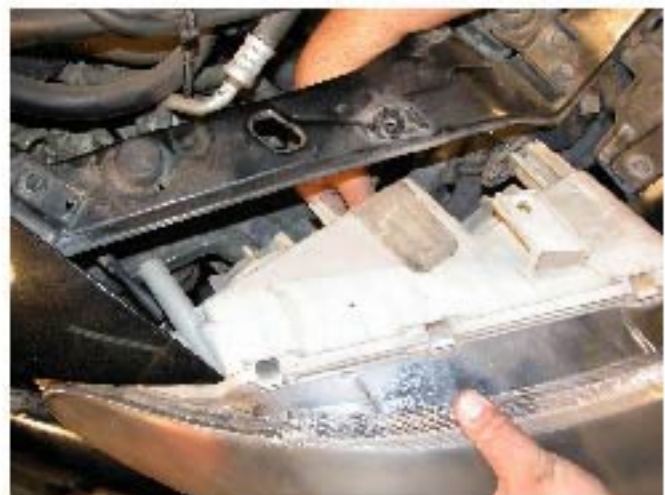
16. Disconnect all the connectors, and remove the headlight
