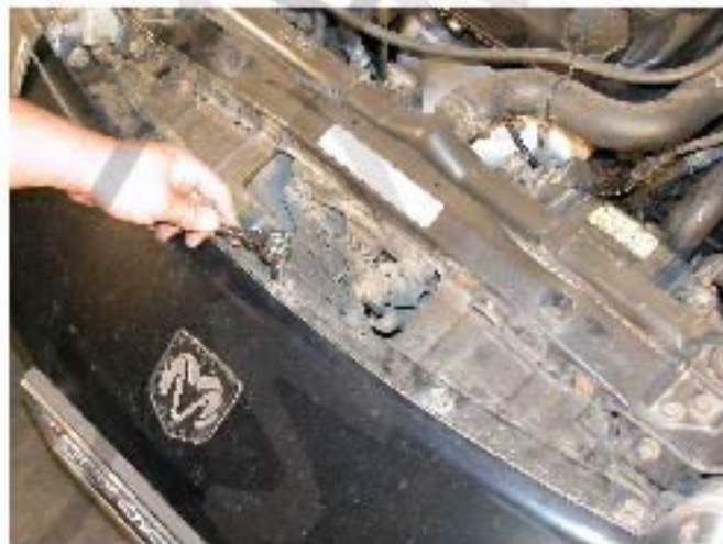
2. Remove the bolts from top bumper first
