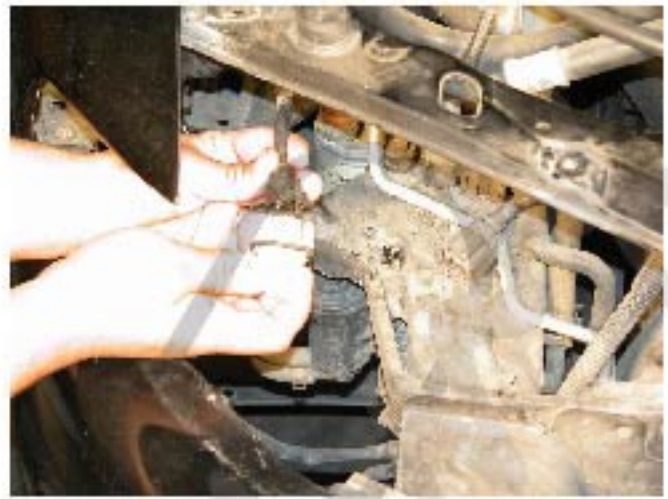
18. Connect the driving light socket back to the wire which is located inside the vehicle
