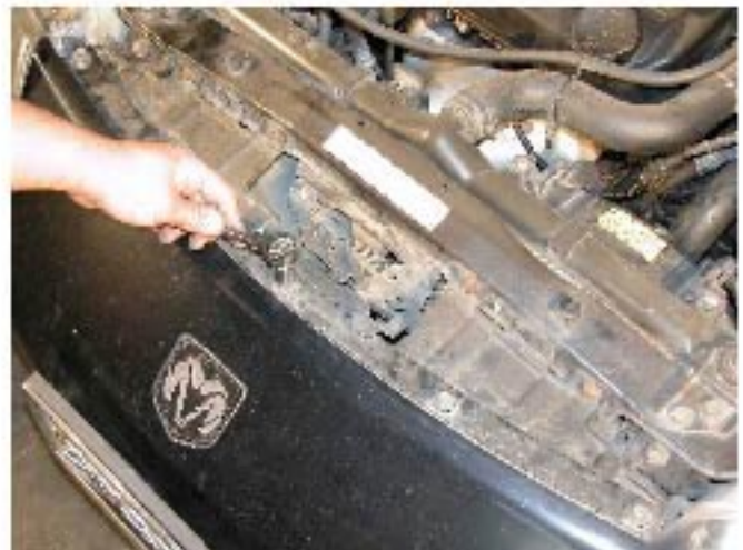
28. Install the five 10mm bolts
