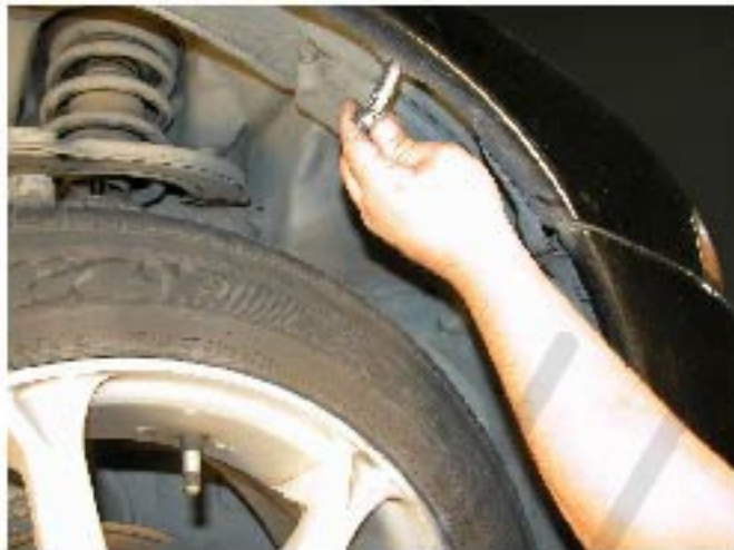
7. Next to the suspension, there are 10 mm bolts that need to be removed
