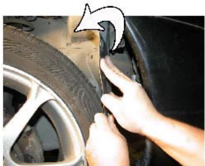
10. Then gently pull the plastic cover just enough to see the inside of bumper
