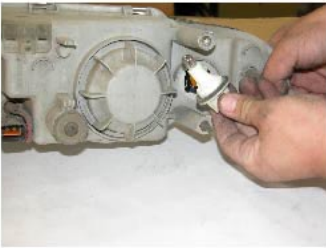
17. Take out the driving light socket from OEM headlight
