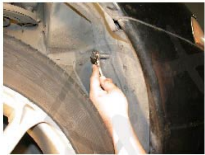
6. Remove the two bolts
