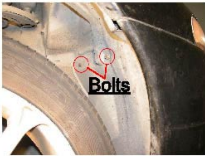
5. There are two bolts next to the three clips
