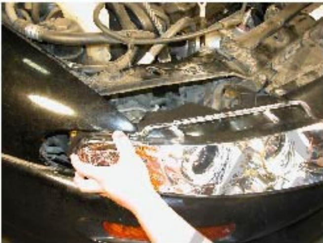
19. Install the headlight to the original spot
