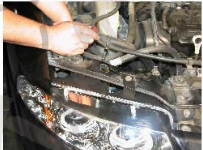
20. Install the bolts on the outer side of the headlight first
