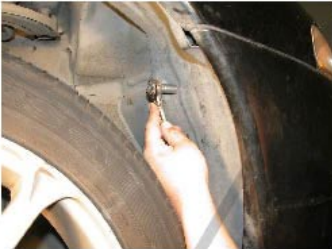
25. Install two 10mm bolt
