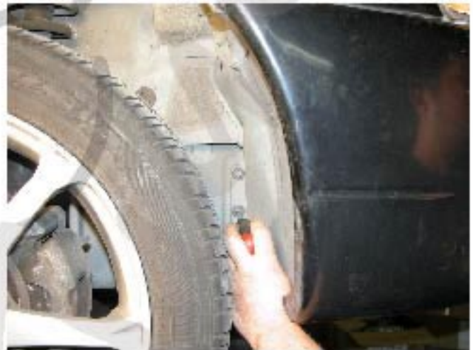
26. Install the two clips
