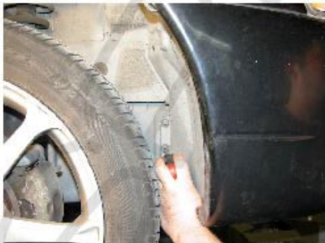
9. Remove the two clips first
