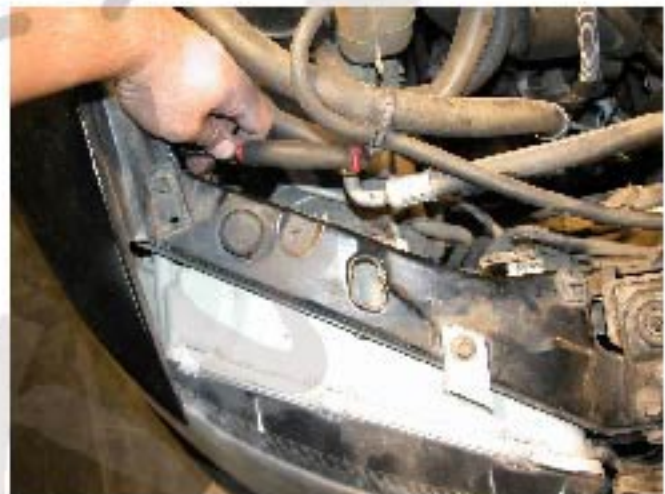
14. Remove the three bolts
