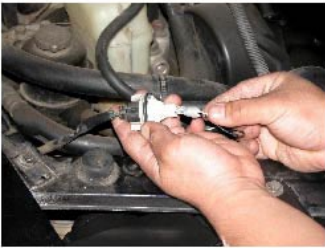
23. Take out the driving light bulb from socket, connect the Halo LED connector in this driving light socket
