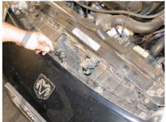
2. Remove the bolts from top bumper first
