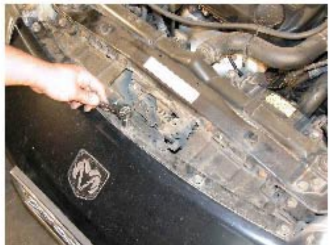
28. Install the five 10mm bolts
