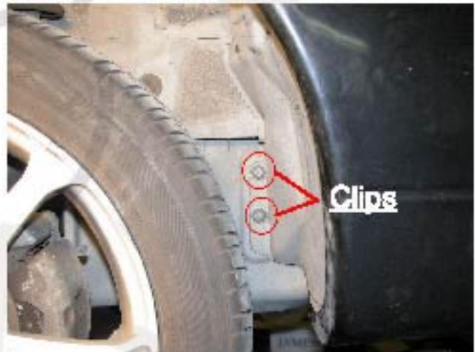
8. Under the two bolts, there are two clips that need to be removed
