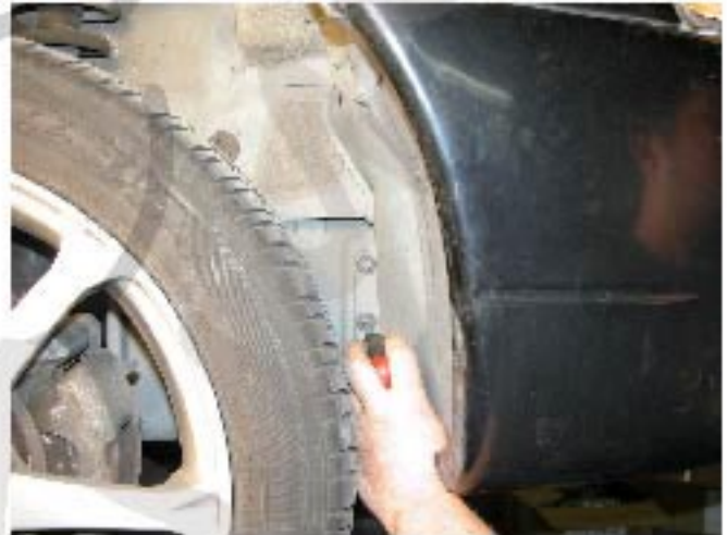
26. Install the two clips
