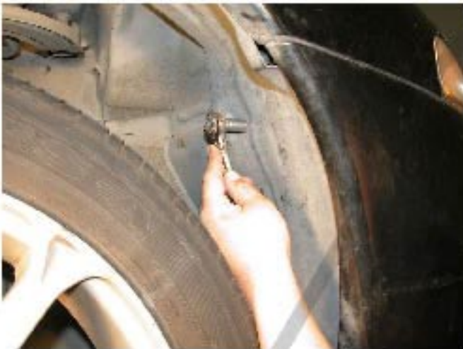
25. Install two 10mm bolt
