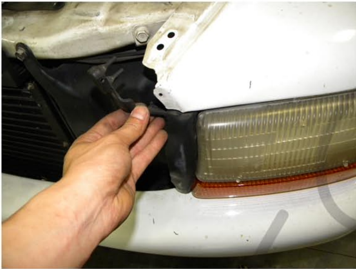
1. Remove the rubber weather seal from fender (1 plastic clip)
