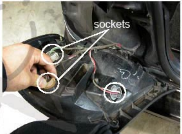
8. Remove all the sockets by turning them counter clockwise to unlock them
