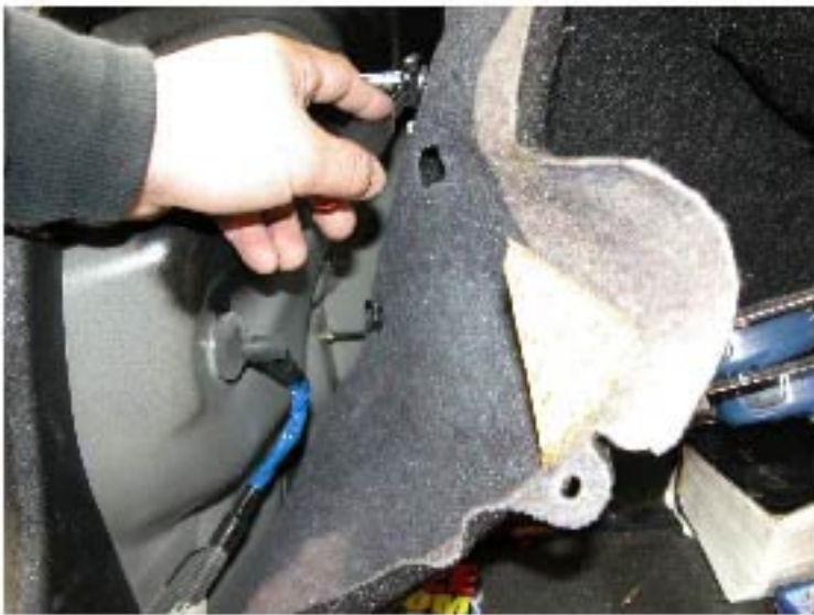
5. Remove the three screws which are inside the plastic cover shown earlier
