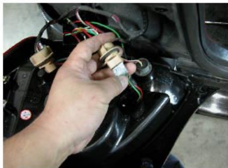
10. Plug the male harness from the L.E.D. tail light to the vehicle sockets by gently pushing them in for a snug fit
