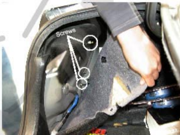
2. Open the plastic cover Inside the plastic cover, there are three screws
