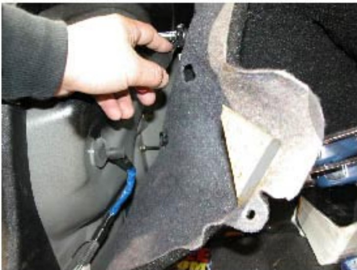
13. Install the three screws to fasten the tail light
