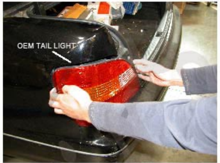
6. Gently pull out the OEM tail light slightly, just enough to see the back of the lights
