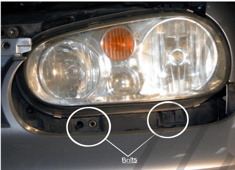
13. Use 8mm socket to remove the two bolts from the bottom of the headlight
