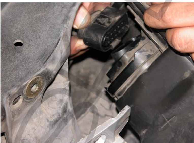
15. Disconnect the harness from the headlight
