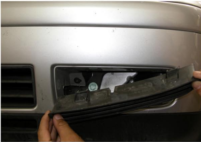
23. Put the plastic cover back on
