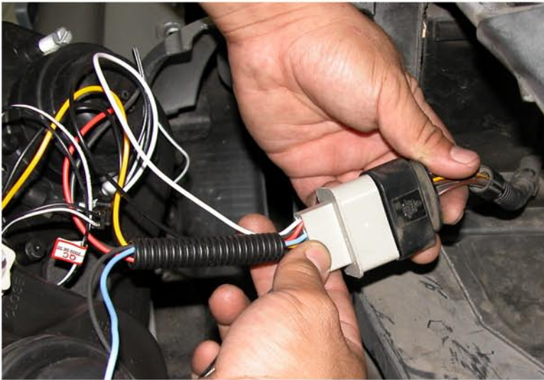
17. Connect the harness from the headlight please see the "Halo and L.E.D.installation instructions" If your headlights don't have HALO or L.E.D. You can skip the installation instructions.
