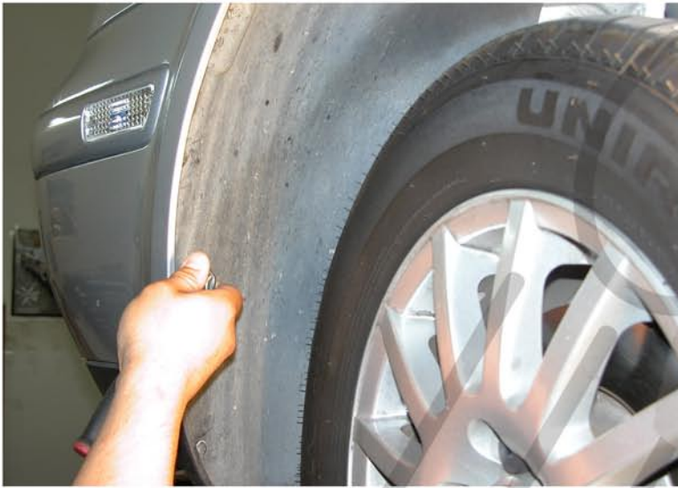
25. Use T25 torx socket to install the bolts to fasten the bumper
