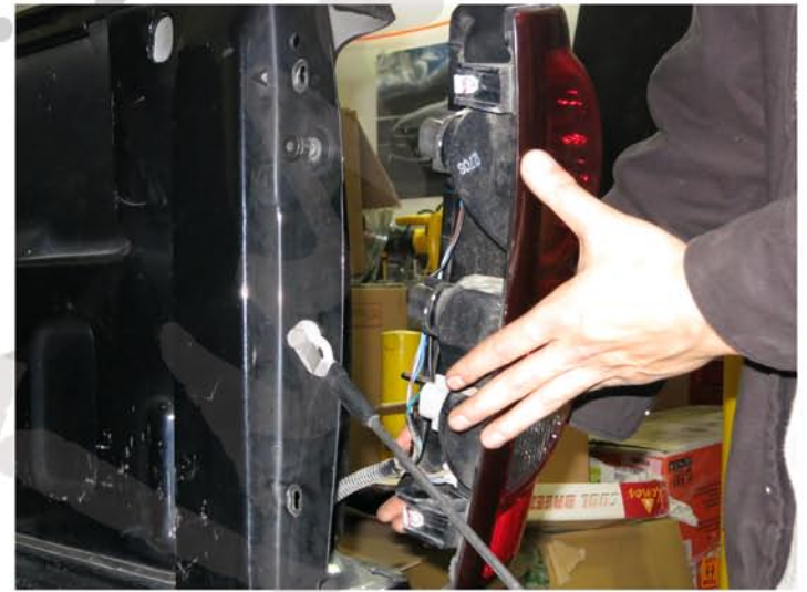
8. Replace the taillight
